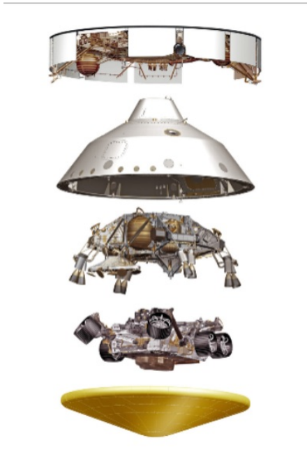
3D rendering of major Mars 2020 spacecraft parts in an expanded view: cruise stage, backshell, descent stage, rover, heat shield.
