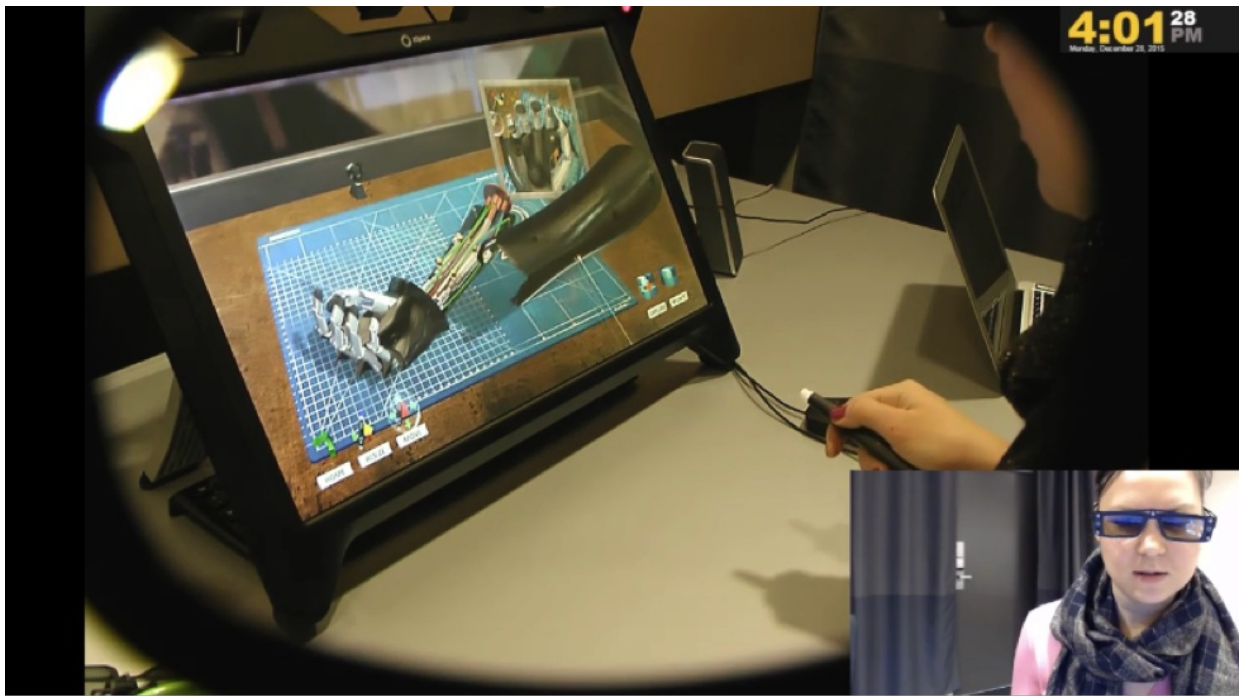
Figure 3. A participant pulling the stylus away from the screen to move part of a mechanical arm closer to her.
